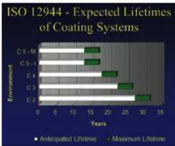
Fig. 3: ISO 12944 - a comprehensive corrosion protection standard. Examples: atmospheres; moderate sulphur dioxide levels; production areas with high humidity; chemical processing plants. C5-I: Industrial areas with high humidities and aggressive Marine, offshore, coastal areas with high salinity.
